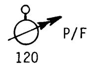
Fixed manually operated dry powder unit with one hose reel
