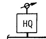
Hydrant post (pillar) double equipped with bottom drain valve
