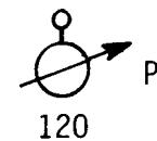
Fixed-installed monitor, remotely adjustable and operated, for powder and for foam (capacity in m<sup>3</sup>/h water foam solution)
