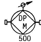
Fixed manually operated AFFF unit with one hose reel and monitor (capacity in m³)
