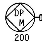
Fixed manually operated dry powder unit with two hose reels and powder gun (capacity in kg)
