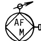
Fixed installed high back pressure foam generator
